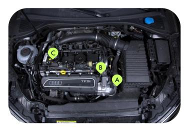
**Harness Section A – Turbo Boost Pressure Sensor –** Route section A down under the airbox and towards the front of the engine, Disconnect the turbo boost pressure sensor connecter and wire in series the PCM wiring harness section labelled A. See figure 3a for assistance.
