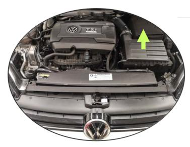
**Stage 3 –** With the airbox pipes and screw removed you are now ready to remove the standard airbox, start by pulling up the air filter box shown in attached image until the airbox is removed from the rubber mounting bobbins. One loose, carefully remove the airbox and place aside.
